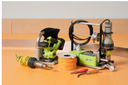
1. The joints are milled out or cut open centrally with an electric milling machine and/or the joint cutter.
