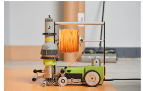
5. The processing temperature is 350-400° C (for noracare™ max. 300 °C). When using a welding machine to process the hot welding rod, set the speed to 2 linear metres/minute. The operating speed and temperature setting can be adjusted on most welding machines.
